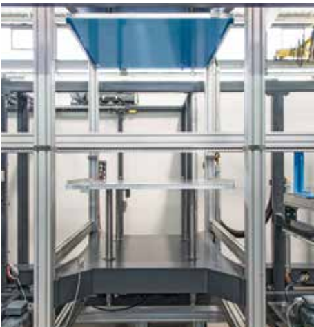
Slug-removal station (e.g. Euro-holes)
