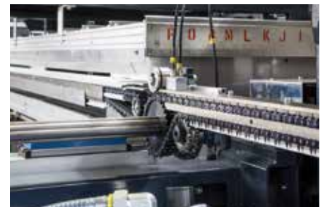
Two step film feed: Optimal provision of the film in the forming station
