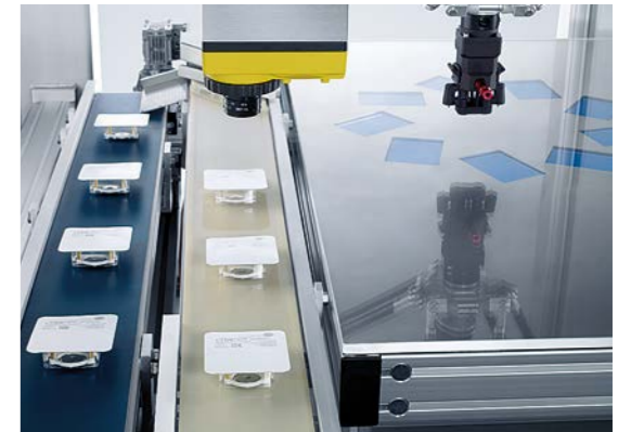
Example of a camera system for the verification of variable product data
