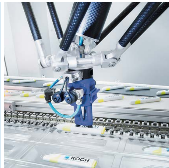
Pick-and-place with maximum servo-regulated precision
