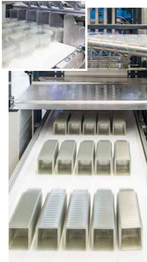
Tip-stacking: easy, manually or automatic packing
